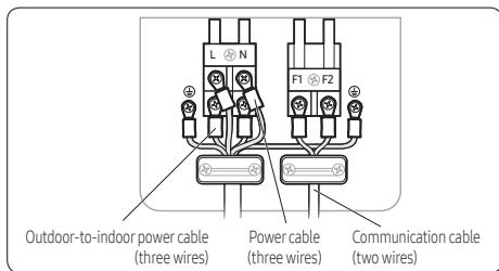
11 Connect the outdoor unit power supply cable to the preinstalled disconnect switch.
