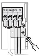
3 In Step 2-2, step 3 you determined the exit position for the piping bundle. If using the left, right, or bottom exits, pass the cables through the selected knockout.
