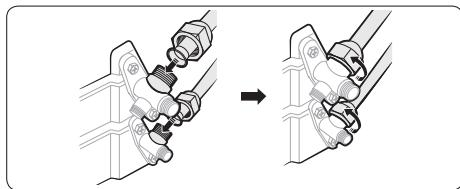
9 Torque the flare connections to the values in Step 2-3, step 7 on page 16.
